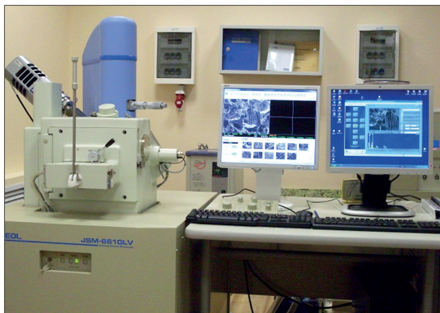
Fig. 1. External view of the scanning electron microscope JEOL JSM-6610LV
