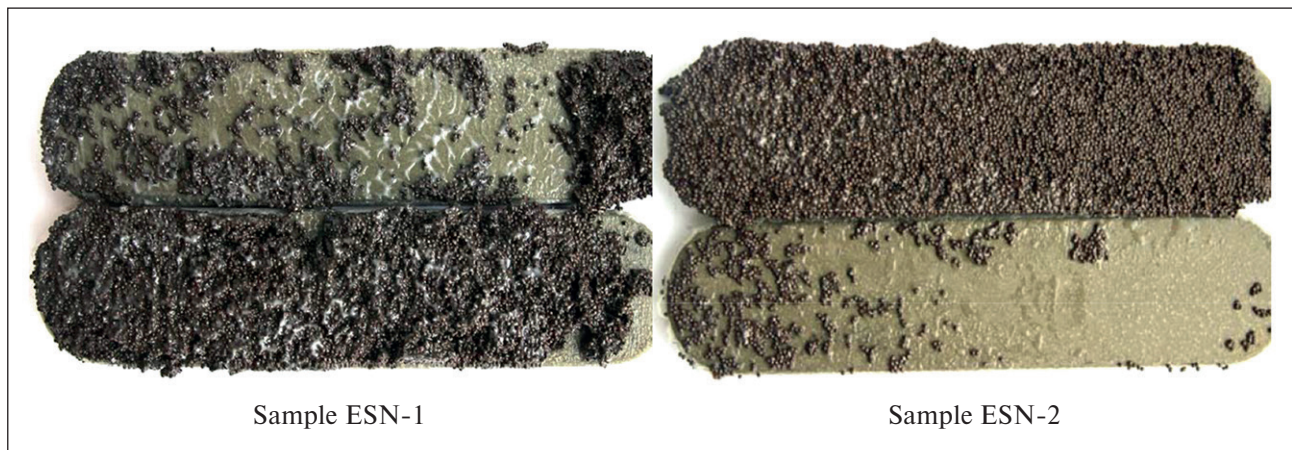
Fig. 2. Visual appearance of ESN-1 and ESN-2 inside the disassembled hydraulic fracture models
