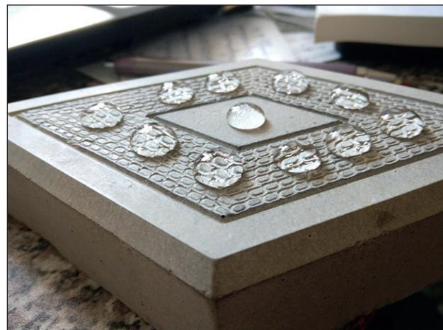
Fig. 7. Paving slabs made of vibrocast concrete with the only silica sol «Флюкс-1ГФ» – only 25 grams of end product per 100 kg of cement
