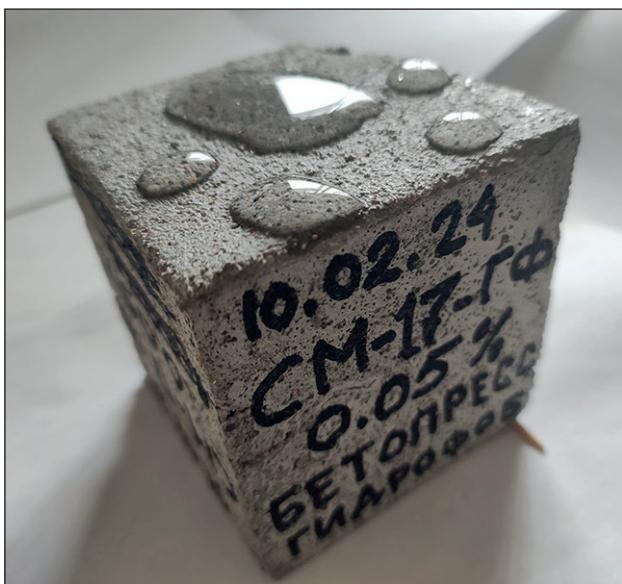
Fig. 2. Vibropressed block made of low-slump concrete on lyophobic sol «ВИБРОФИНИШ СМ-17-ГФ», consumption 0.05% to the weight of cement after 10 days of hardening
