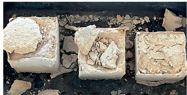
Fig. 14. Breakdown of the ceramic composite obtained by semi-dry pressing
