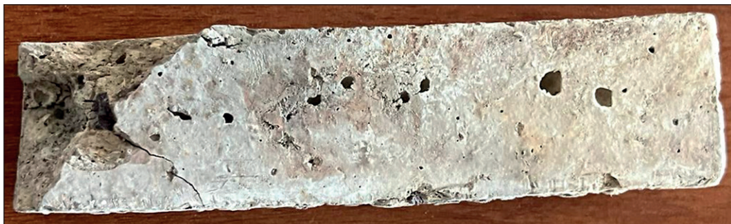
Fig. 13. Failure of the ceramic composite with 50% barite powder content
