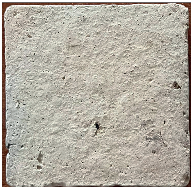
Fig. 15. Ceramic composite: bentonite – 90%, cavitation-treated barite powder – 10% (firing temperature – 800 °C, firing time – 30 minutes)
