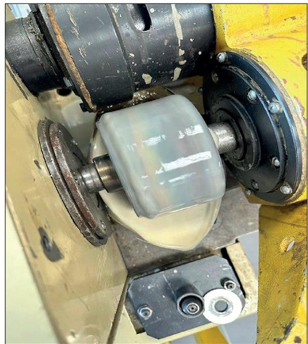
Fig. 3. General view of the modernized friction unit of the AI-5018 machine for testing in the drilling fluid environment
