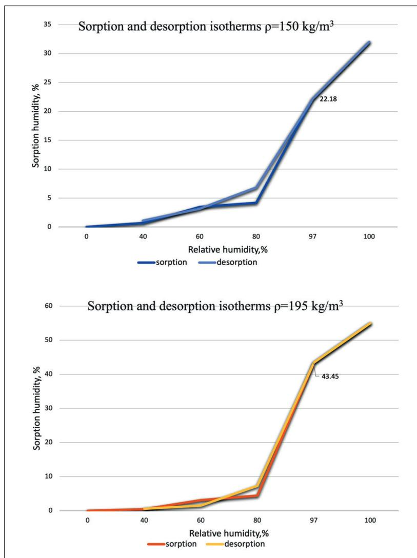
**Fig. 4. Graphs of the sorption and desorption activity of the material based on foamed liquid glass**
