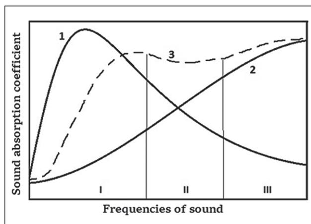
Fig. 1. **The mechanism of sound absorption:** I – resonant sound absorption; II – mixed sound absorption (transitional); III – sound absorption due to friction losses; 1 – sound absorption in the material, due to the characteristics of the matrix; 2 – sound absorption in the material, due to the parameters of its porosity; 3 – integral curve of sound absorption
