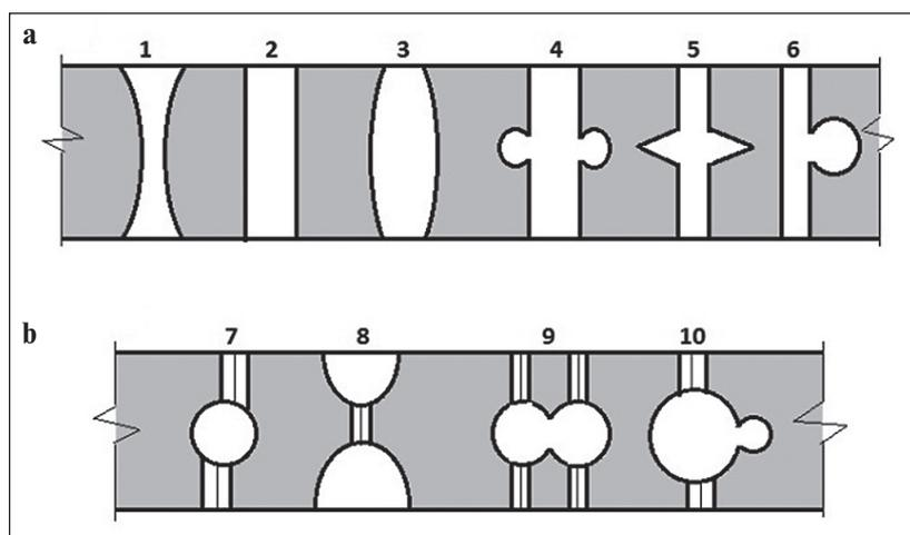
Fig. 2. **Types of pores:** a – open pores; b – closed pores; 1, 2, 3 – types of acoustically active pores; 4, 5, 6, 8 – types of acoustically semi-passive pores; 7, 9, 10 – passive porosity
