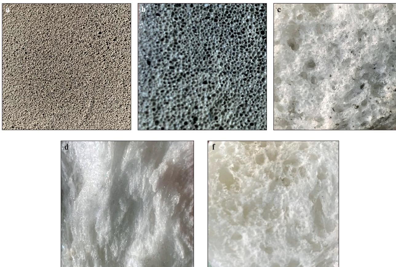
Fig. 3. Structure of various silicate compositions of porous materials: a – foam glass; b – foam glass crushed stone; c – material based on liquid glass with the addition of Portland cement; d – material based on liquid glass and organosilicon additive; e – material based on liquid glass and additives – calcium hydroxide
