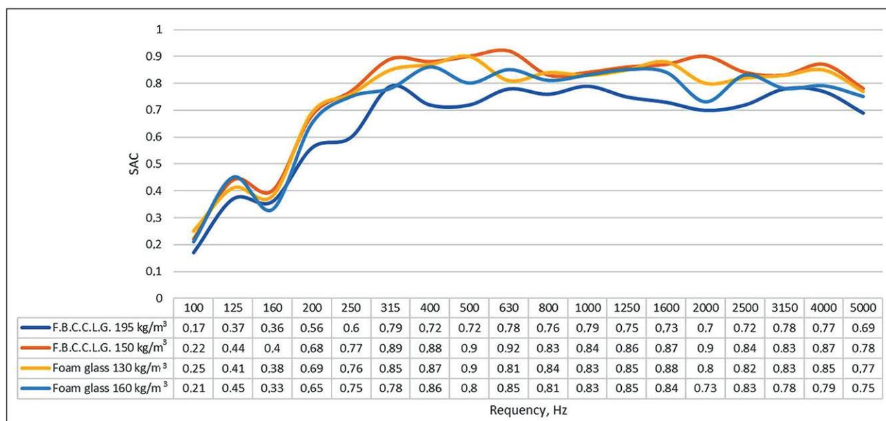
Fig. 7. Test results for determining the sound absorption coefficients of foam glass and materials based on foamed liquid glass
