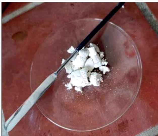
Fig. 1. Photo of bismuth titanate additive immediately after synthesis
