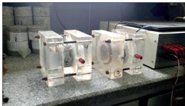
Fig. 6. Rapid chloride penetration test setup
