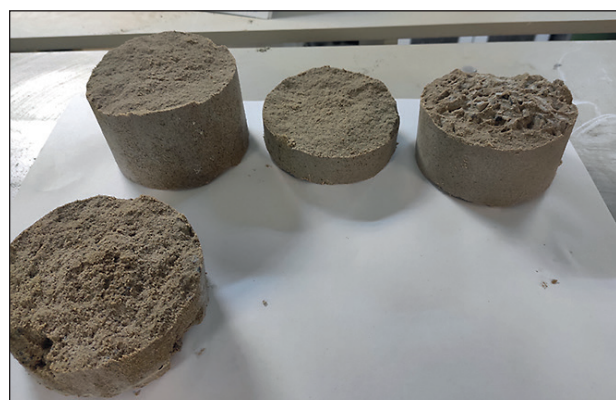
Fig. 6. Uniaxial compression test of a cut core of stabilized soil
