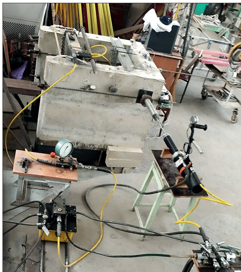
Fig. 2. Testing of an experimental reinforced concrete model (the process of tensioning basalt composite reinforcement is shown):
