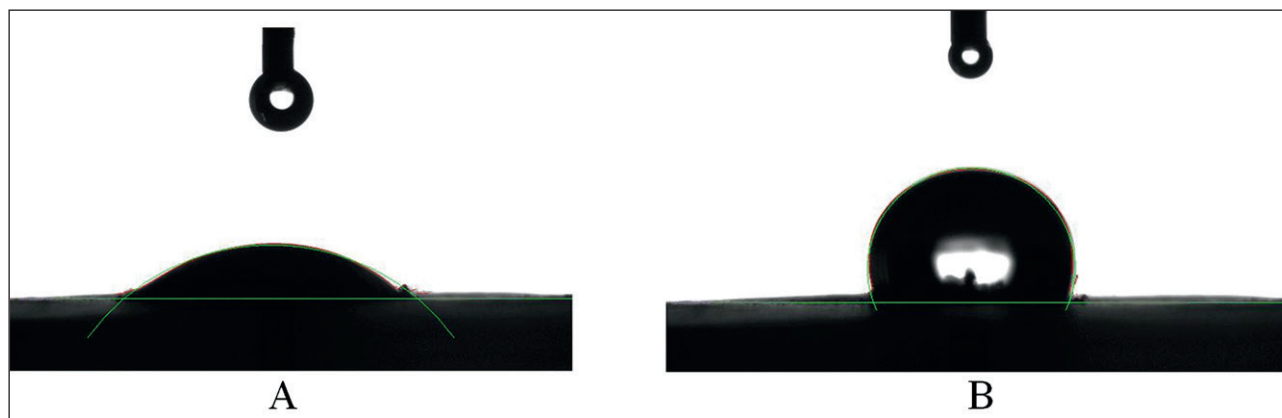
Fig. 3. Water drop on the surface of fine powder: A) 604 nm fraction (grinding time 5 min); B) 314 nm fraction (milling time 30 min)
