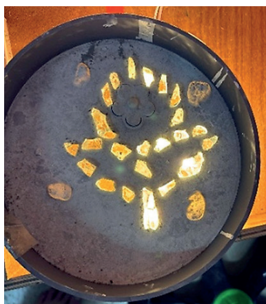
Fig. 13. Preparation of molds and casting of the concrete mixture for product molding
