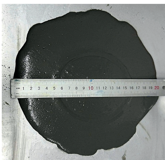
Fig. 14. Measurement of the slump flow of concrete mixtures
