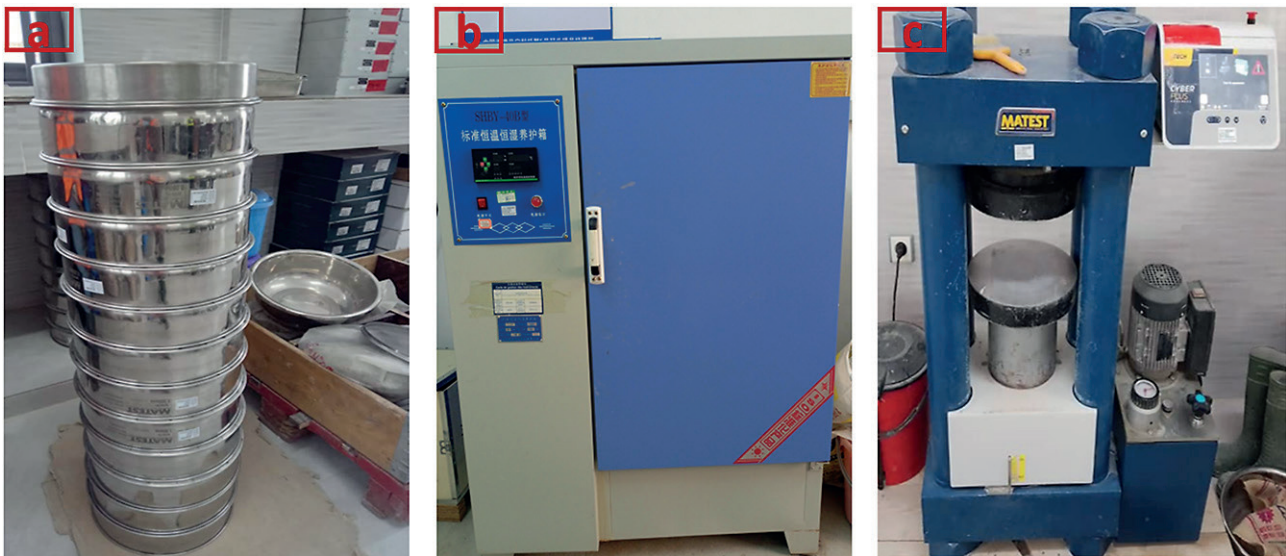
Fig. 3. a – Series of sieves; b – Oven; c – Compression testing machine
