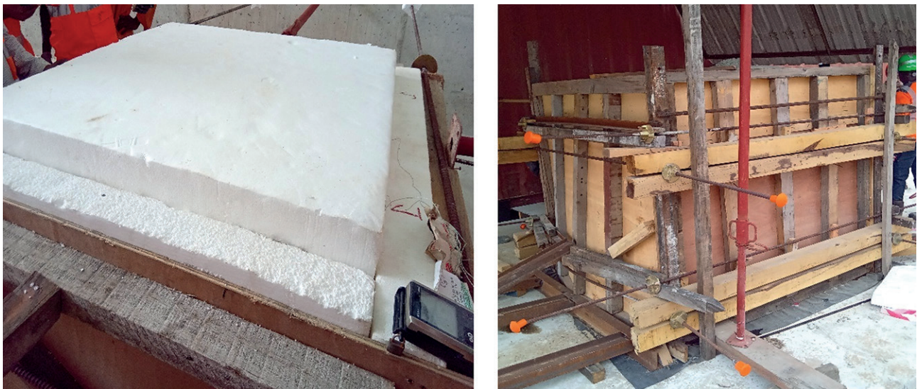
Fig. 7. On the left: DEF cube 1×1×1 m 3 , and on the right: DEF cube 1.6×1.6×1.6 m 3
