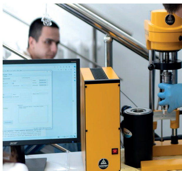
Fig. 7. Determination of the dynamic viscosity of the sample
