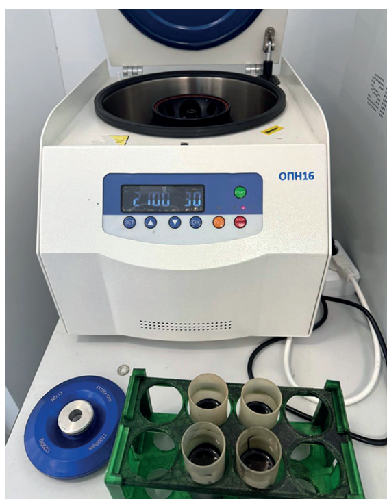
Fig. 2. The process of separation of the emulsion by centrifugation
