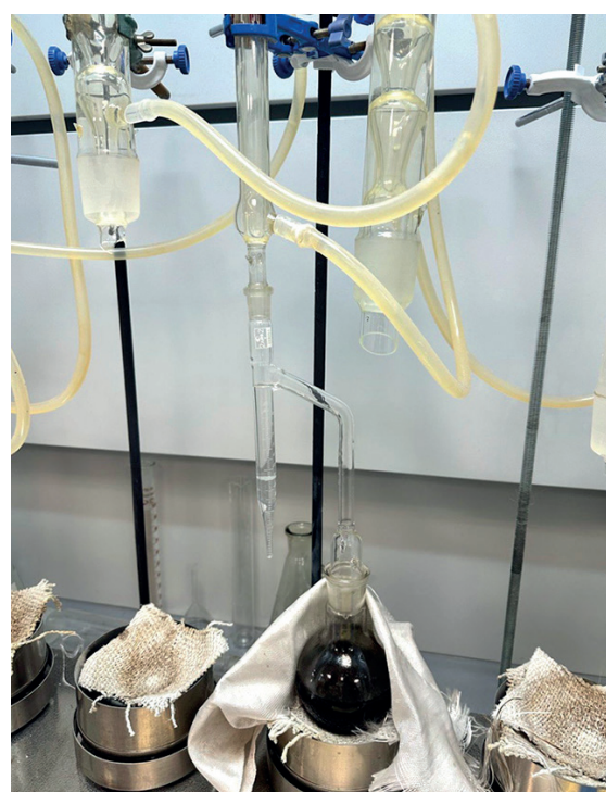
Fig. 3. Determination of water content by the Dean-Stark method
