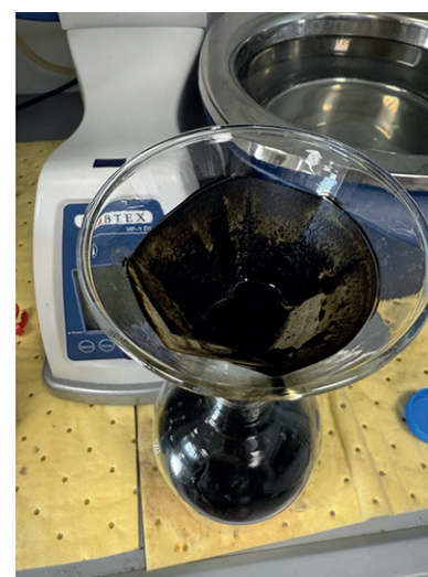
Fig. 9. The process of extracting the oil component from the “Large Pond point # 2 (+3.3 m mark)” sample
