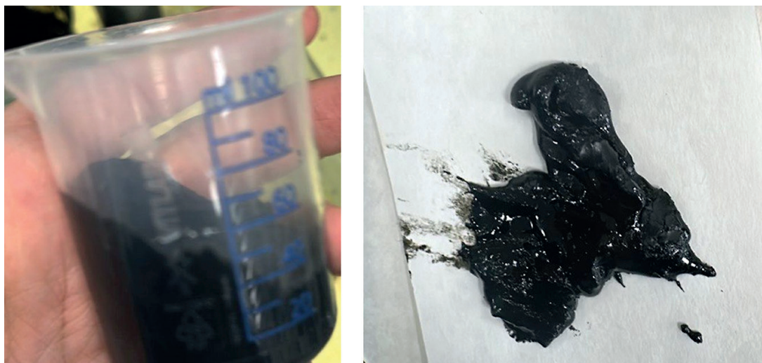
Fig. 12. Sample appearance after centrifugation of the “sample + diesel fuel” mixture
