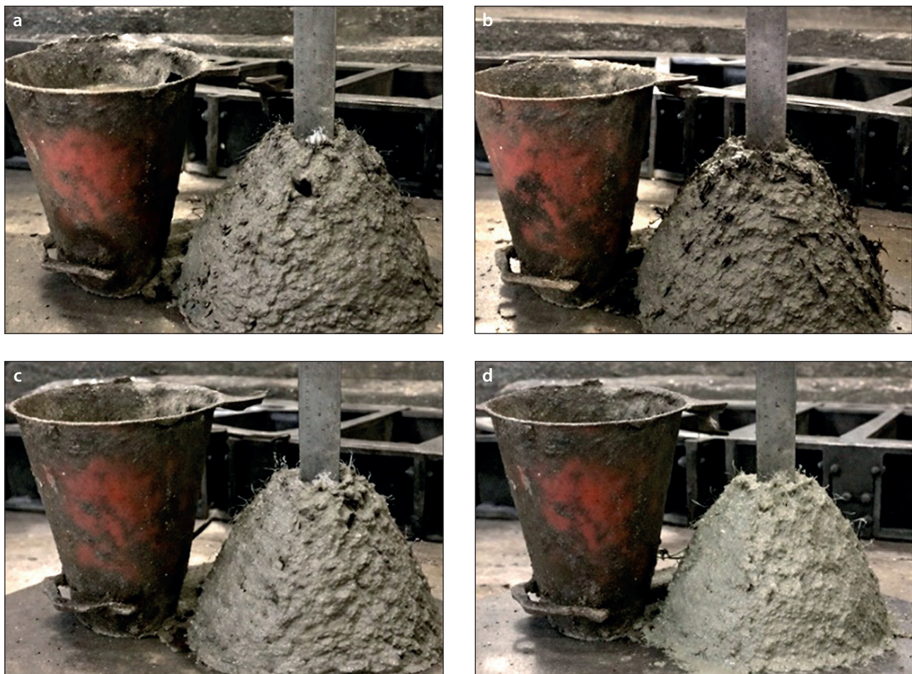
Fig. 5. Appearance of the concrete mixtures after the slump test: a – mixture with steel fiber; b – mixture with basalt fiber; c – mixture with polypropylene fiber; d – mixture with glass fiber
