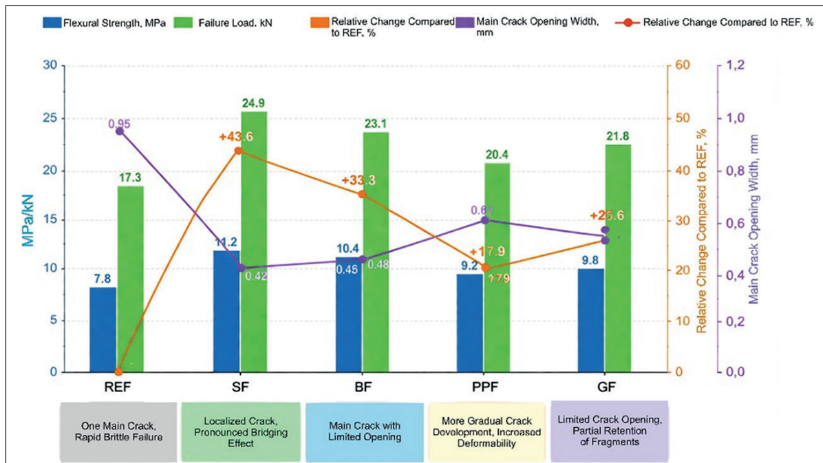
Fig. 12. Comparison of flexural strength and crack resistance of concrete mixtures with different types of fiber reinforcement
