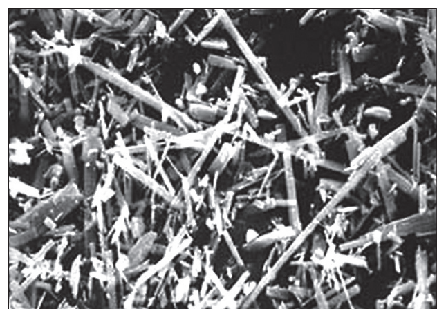
Fig. 2. Microstructure of Wollastonite (magnification ×1700)
