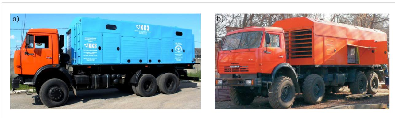
Fig. 10. Nitrogen station TGA-5/10 (a) and fire engine of Krasnodar Compressor Plant (b)
