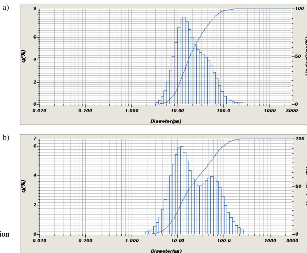
Fig. 1. Size distribution of coke 1 (a) and coke 2 (b)
