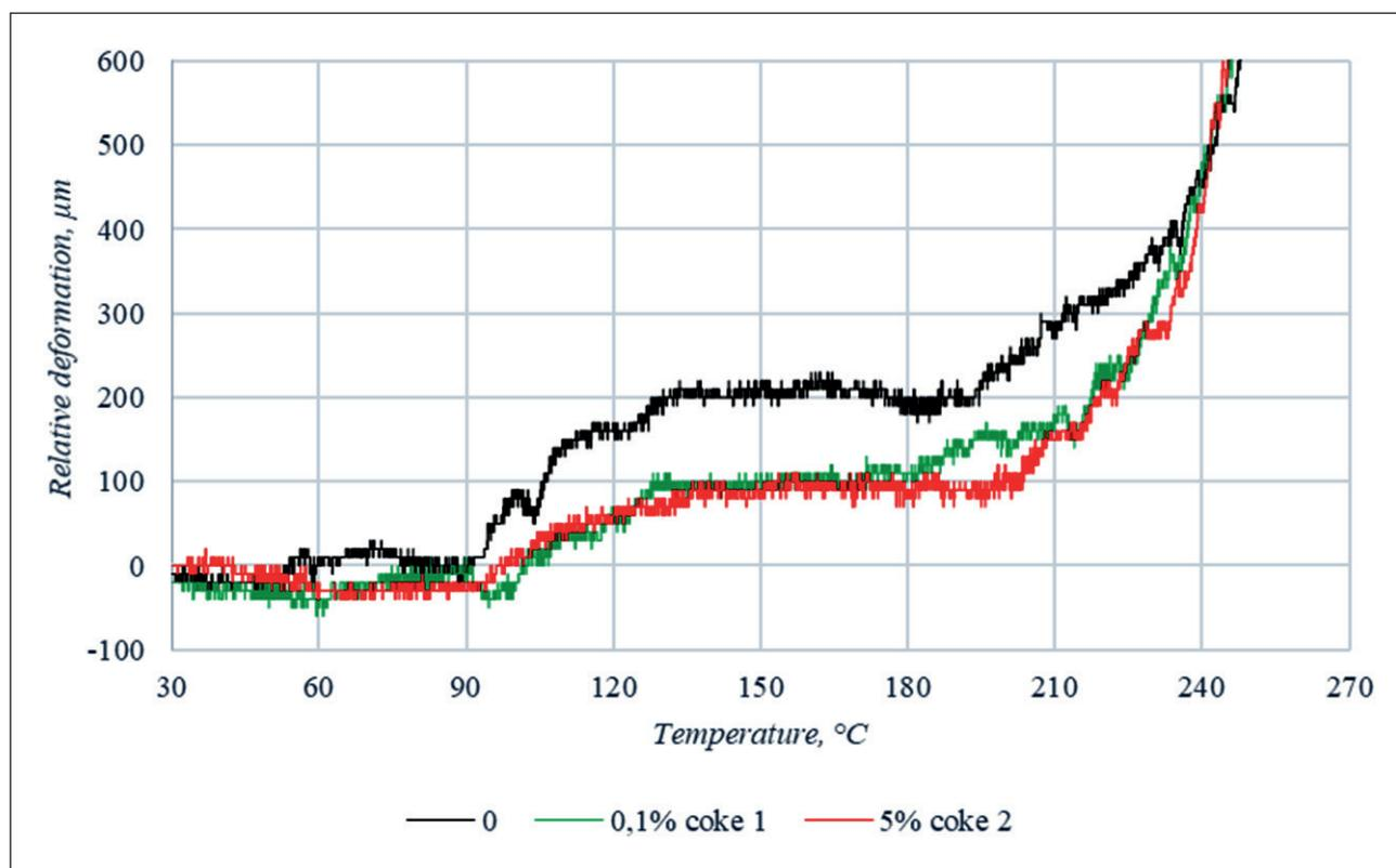
Fig. 3. Thermomechanical curves of PVC-WPC samples (rate of temperature rise 3°C/min, specific compressive load 1N)
