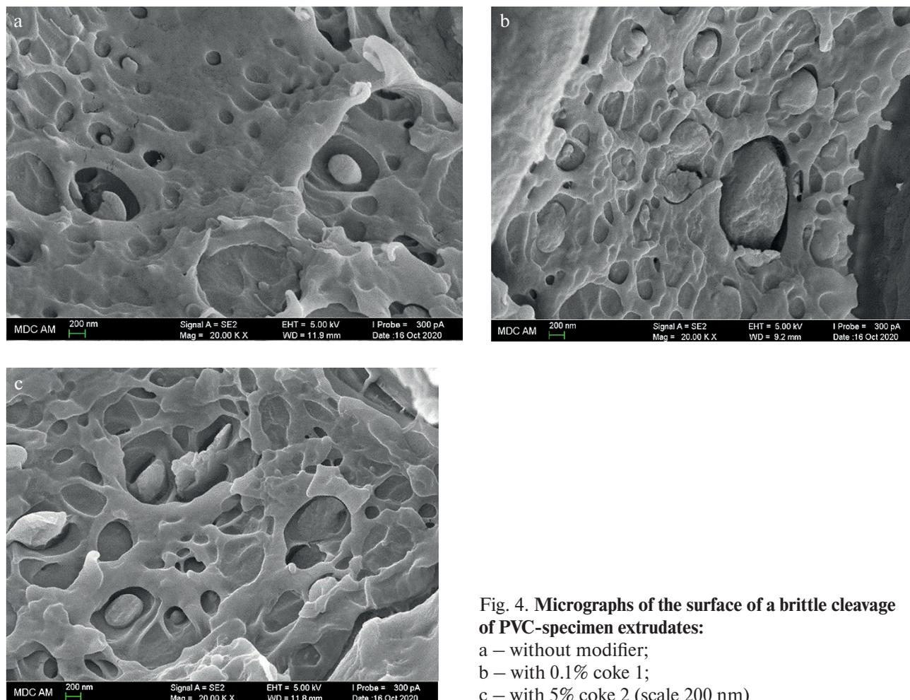
**Fig. 4. Micrographs of the surface of a brittle cleavage of PVC-specimen extrudates:**
