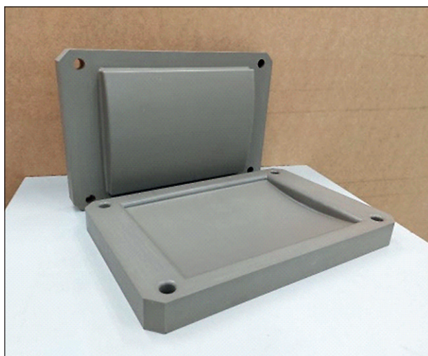
Fig. 7. Low pressure mold made from polymeric materials
