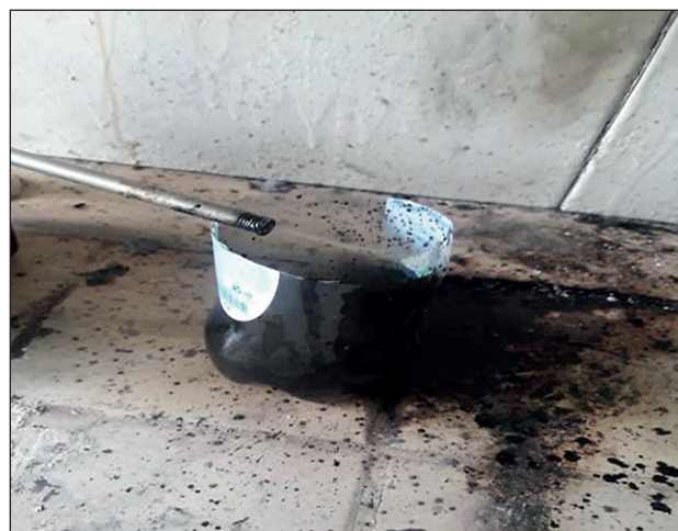
Fig. 2. Pyrogenetic water, resin and gases obtained as a result of coal pyrolysis
