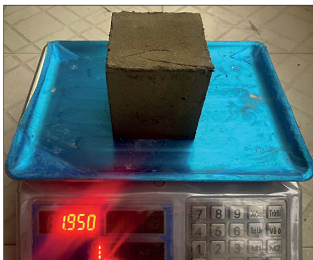
Fig. 12. Determination of the average density of developed concrete at the age of 28 days
