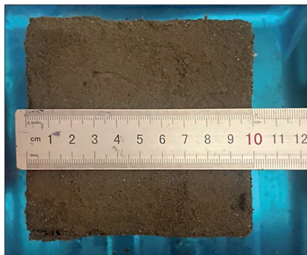
Fig. 12. Determination of the average density of developed concrete at the age of 28 days
