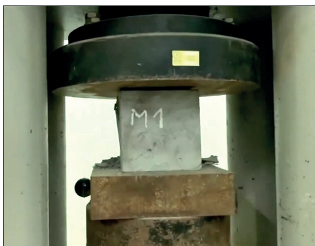
Fig. 10. Compression testing of concrete samples
