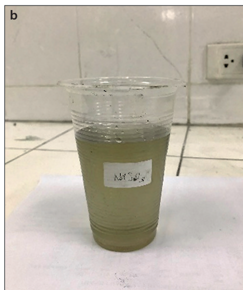
Fig. 8. Activating alkaline solution: a – 10 M sodium hydroxide solution; b – two and a half aqueous sodium silicate solution
