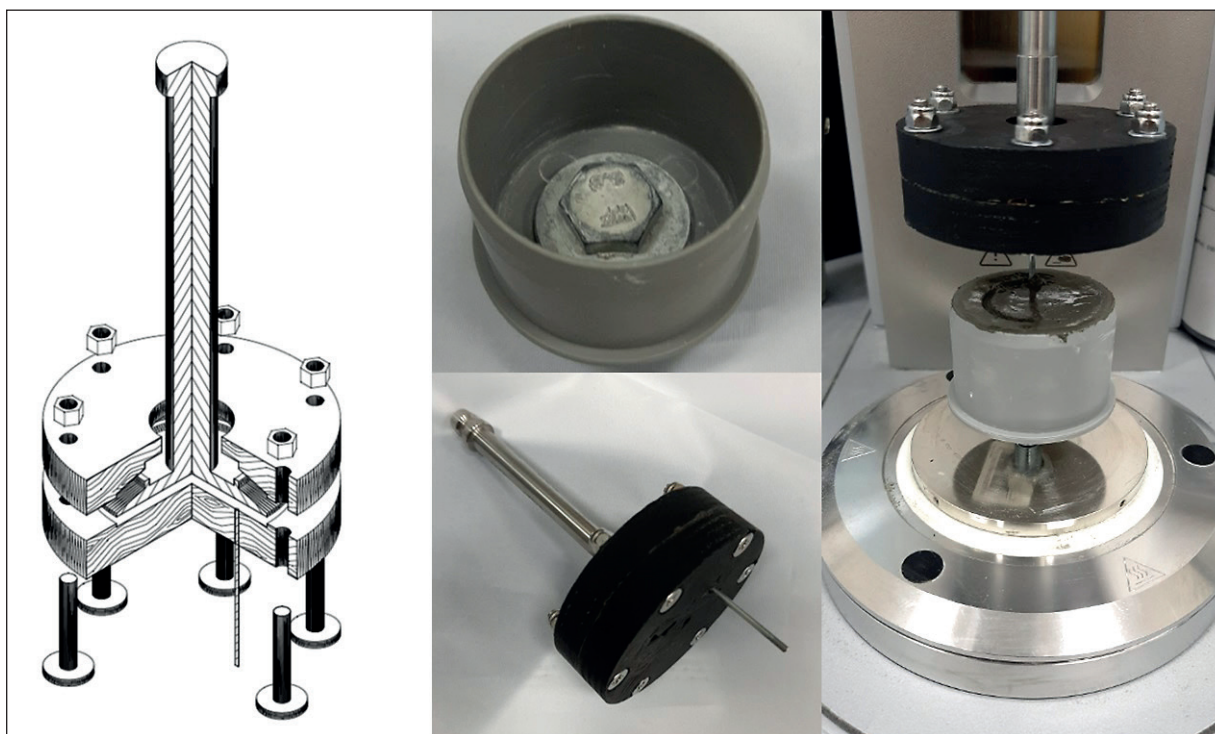
Fig. 2. Diagram and photos of the measuring system for controlling the kinetics of mineral binder setting
