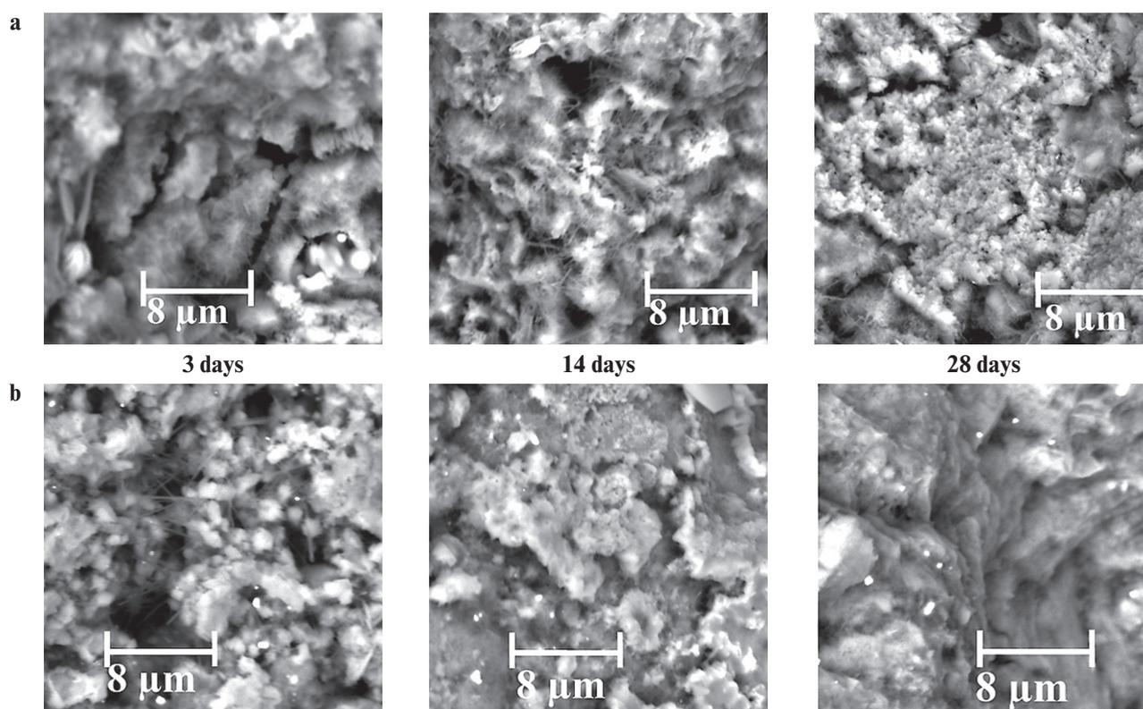
Fig. 8. Microstructure of cement samples from the control composition (a) and modified with a mixture of WC, TiC powders (b) at the age of 3, 14, 28 days
