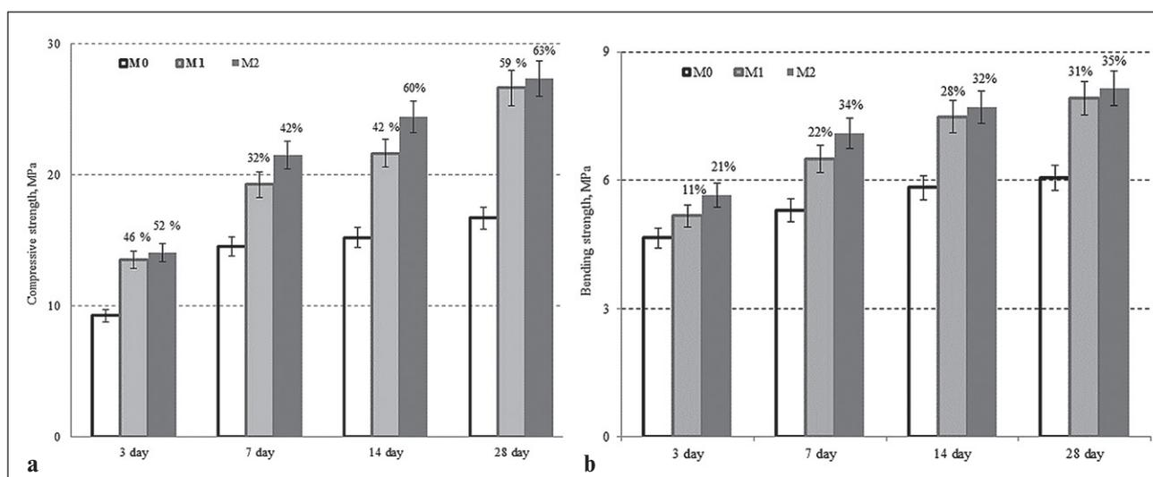
**Fig. 5. Kinetics of strength development in compressing (a) and bending (b) for cement-sand mortar of the composition M0 and M1, M2**
