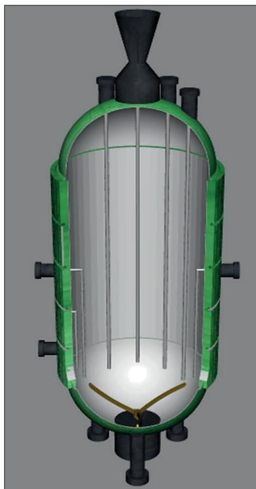
Fig. 5. Polymerization reactor
