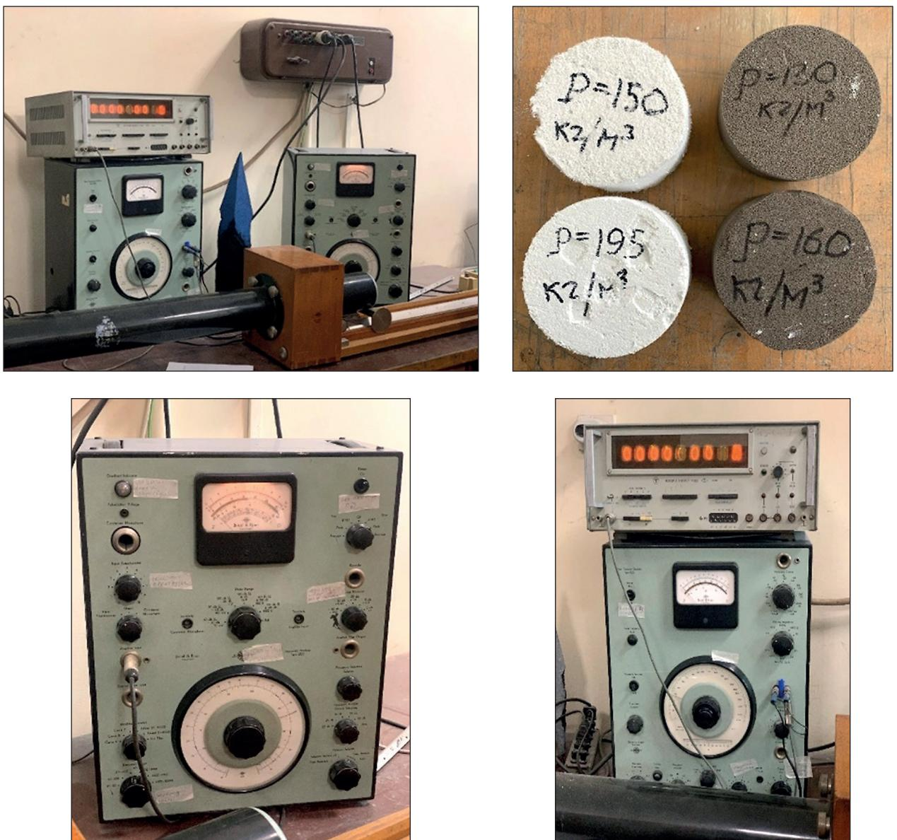
Fig. 6. Sound absorption test apparatus and test material samples
