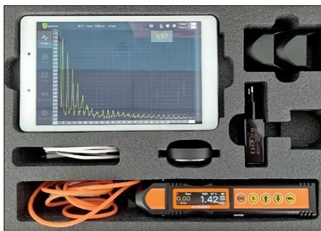
Fig. 3. EMA thickness gauge EM4000
