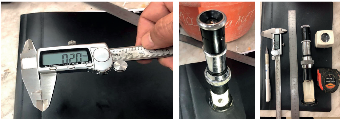
Fig. 5. Equipment for measuring the geometric dimensions of fiber
