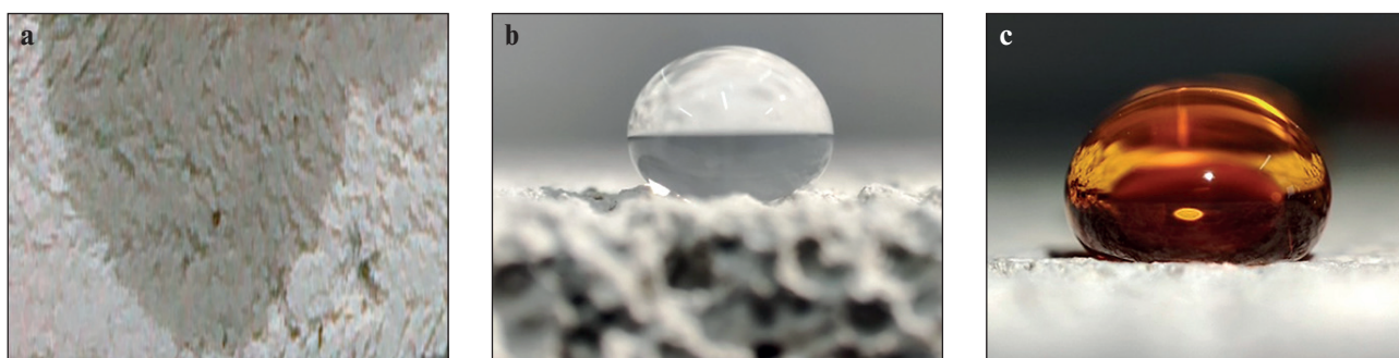
Fig. 9. Image of water drops on an untreated aerated concrete sample (a) and on a sample of aerated concrete treated with a composition based on calcium polysulfide (b), and colored drop (c)
