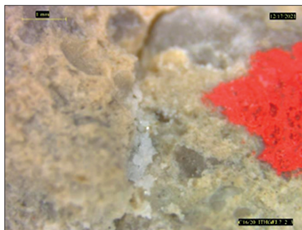
Fig. 3. Concrete sample microphotograph of C16/20BG (additive “Betomix-ITH Gel”, 7 days of hardening) after mechanical destruction and exposure to water for 26 days
