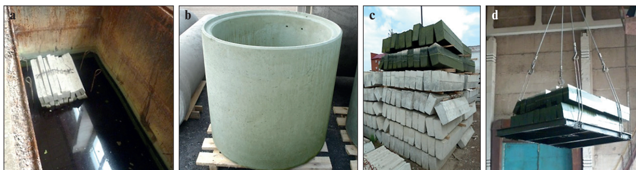
Fig. 11. Scheme of treatment with polysulfide solutions (a–d) for concrete curbs and pipes using an impregnation tank
