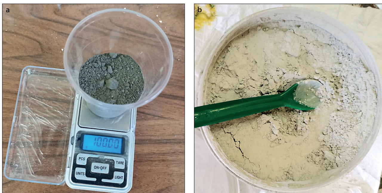
Fig. 4. a) Weighing Portland cement on electronic scales; b) Example of one of the additive components (silicon carbide (SiC) nanopowder)
