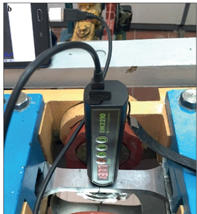
Fig. 2. Installation for testing cyclic load: a – general view; b – control of a metal sample with the EM2210 device
