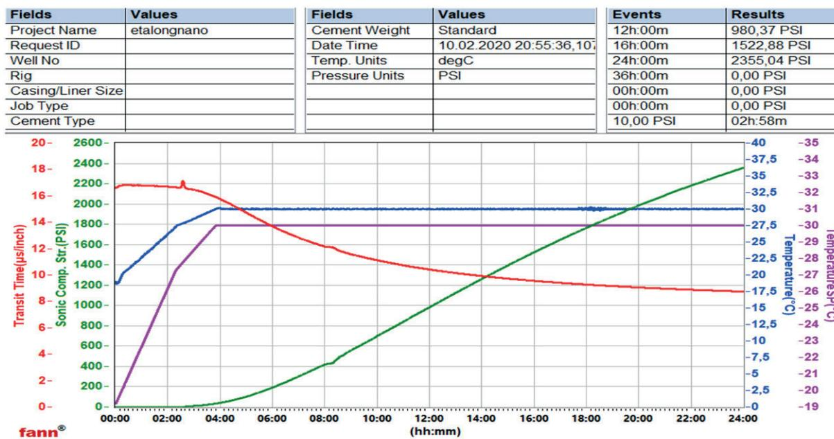
Fig. 1. Change in compressive strength of stone from additive-free Portland cement at 30°C
