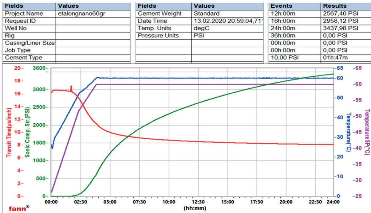
Fig. 4. Change in compressive strength of stone from additive-free Portland cement at 60°C
