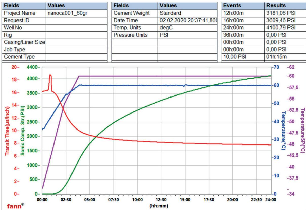
Fig. 5. Change in compressive strength of Portland cement stone with 0.01% calcium carbonate nanopowder at 60°C
