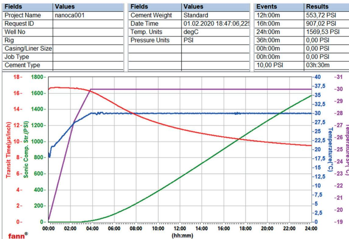
Fig. 2. Change in compressive strength of Portland cement stone with 0.01% calcium carbonate nanopowder at 30°C
