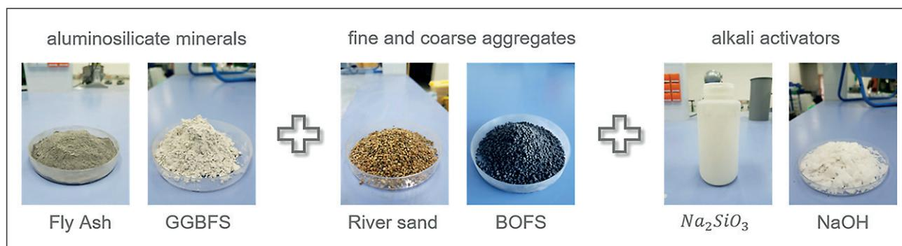
Fig. 1. Composition of geopolymer concrete
