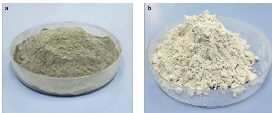
**Fig. 3.** Class F fly ash (a) and ground granulated blast furnace slag, GGBFS (b)
