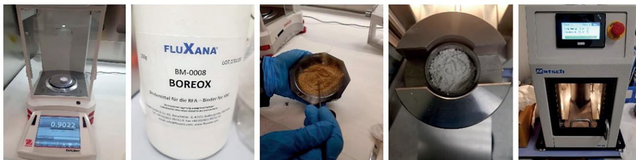
Fig. 5. Procedure for preparing a pelletized sample for X-ray fluorescence (XRF) analysis
