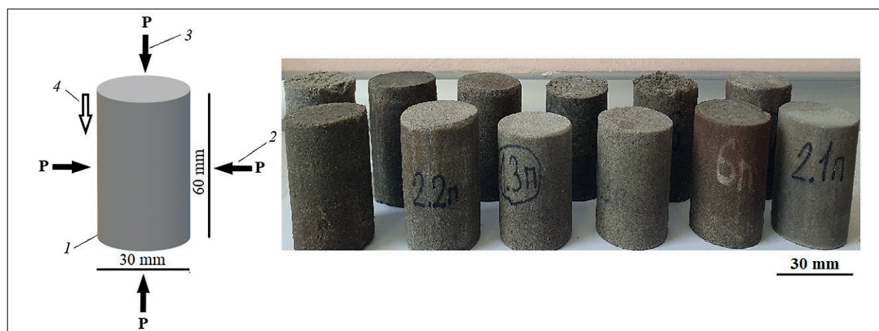
Fig. 3. Geomaterials for filtration experiments. 1 – cylindrical sample of geomaterial; 2, 3 – lateral and axial compression of samples by external pressure; 4 – direction of gas filtration
