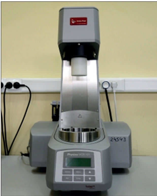
Fig. 1. MCR 101 rotational viscometer with a ball measuring system
