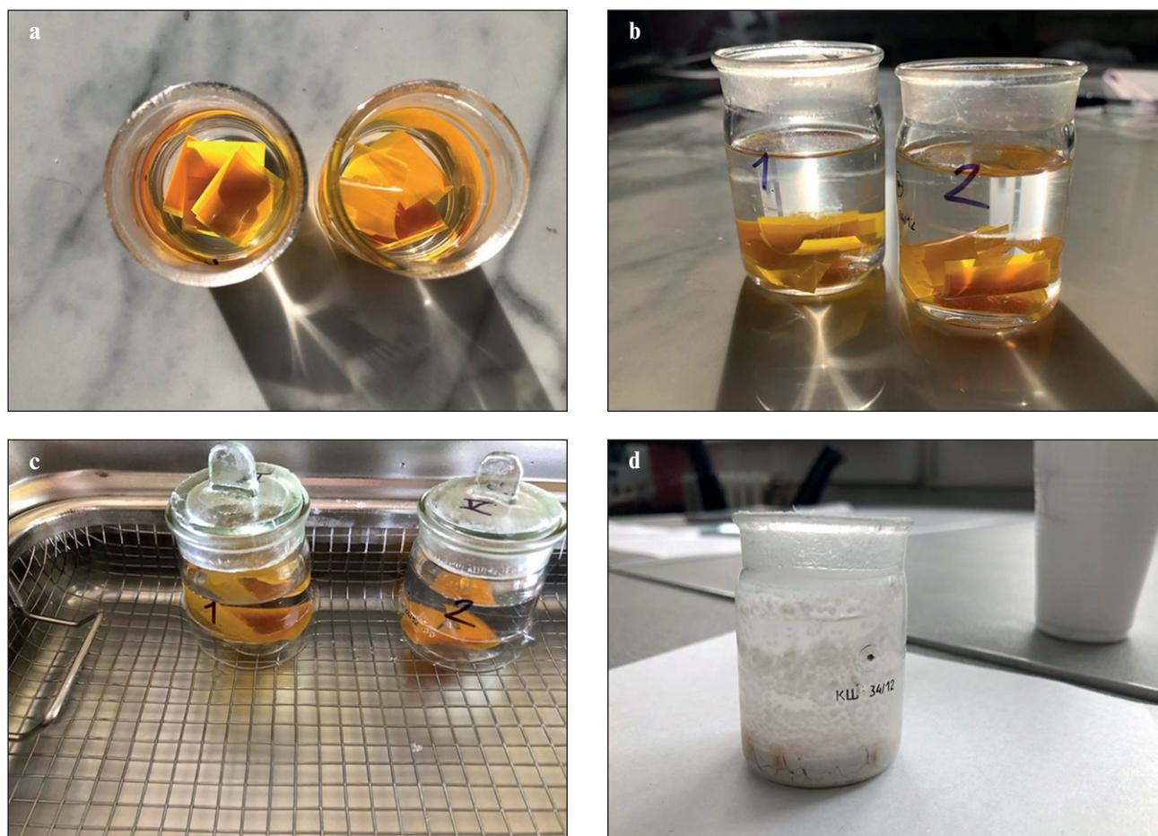
Fig. 2. The process of hydrolysis. Sample preparation (a, b), hydrolysis process (c), hydrolysis result (d)
