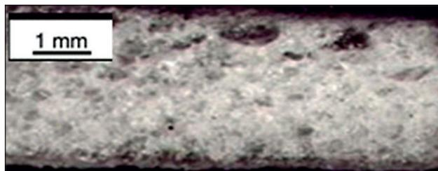
Fig. 4. The cross section of the heat-treated non-woven fabrics based on a mixture of PET (70%) and BCV (30%). Shaft temperature – 180°C (The contact with the metal plate is at the bottom)
