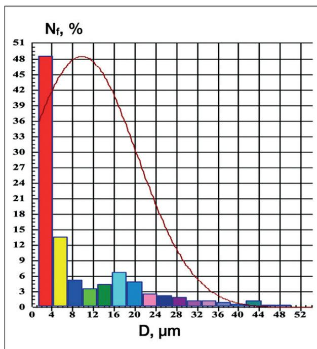
Fig. 6. The metal particle size distribution before the filtration
