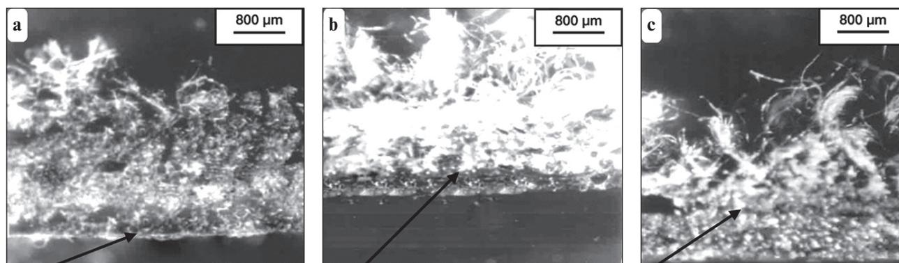
Fig. 2. The cross section of PET (70%) and BCF (30%) based heat-treated fabrics. Processing speed, m / min: a – 15; b – 12; c – 3.5. Shaft temperature – 180°C (The arrows show the boundary between the modified surface layer and the volume)
