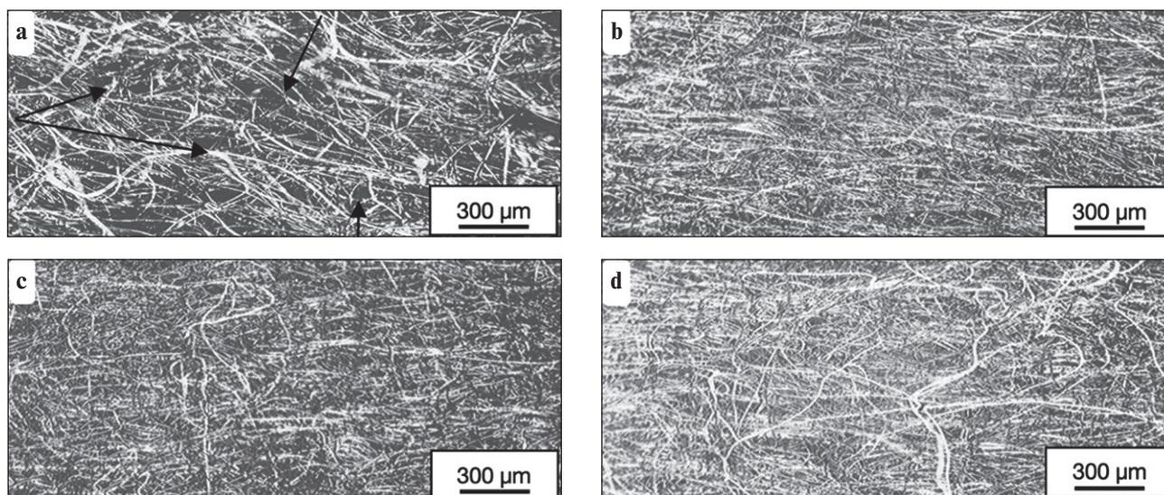
Fig. 3. The surface of the non-woven fabrics based on PET (70%) and BCV (30%) mixture: a – original unmodified non-woven material. Material processed at speed, m/min: b – 15; c – 12; d – 3.5. Shaft temperature – 180°C (Arrows on the surface of the canvas show the holes from the action of the needles, the direction of treatment is shown by the arrows on the side)
