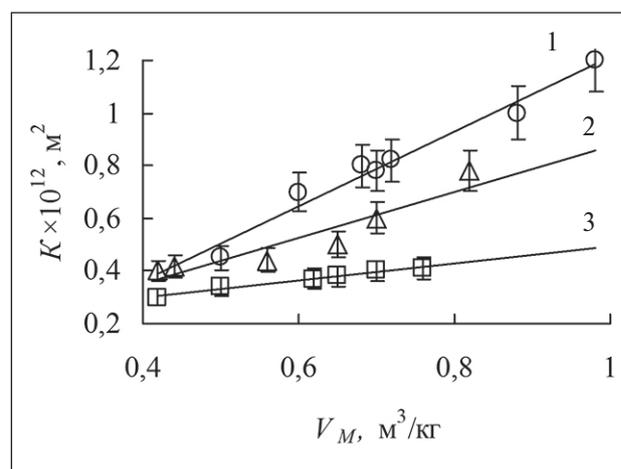
Fig. 5. The dependences of the water permeability coefficient on the specific pore volume of the canvas with different bulk density: 1 – the original unmodified canvas; 2 – the materials heat-treated on the plate for 0.5; 1.0; 3.0; 4.0; 6.0 and 10.0 min; 3 – the materials obtained by processing between the shaft and the conveyor belt at the speed of 3,5, 12 and 15 m/min. The heat treatment temperature – 180°C
