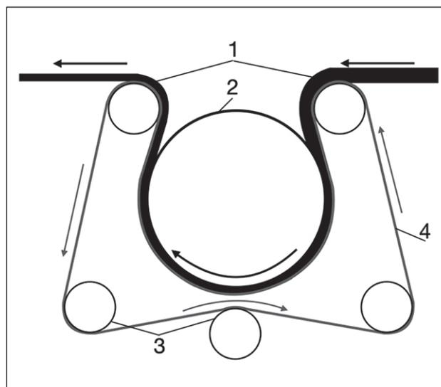
Fig. 1. The scheme of the equipment for the non-woven fabrics deformation-heat treatment:
