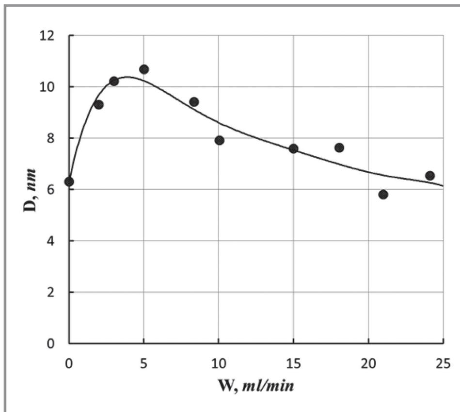
Fig. 12. The dependence of the silica sol nanoparticle size, on the feed rate of the feeder.
