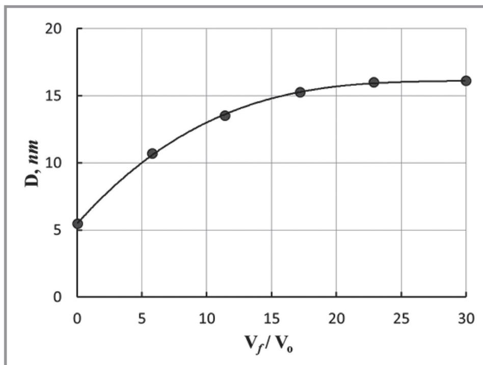
Fig. 13. The dependence of the nanoparticle size silica sol on the ratio  $V_f/V_o$ .
