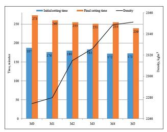
Fig. 3. Cement paste setting time results
