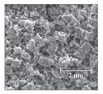
Fig. 1. Micrograph powder mixture of tungsten carbide and titanium carbide
